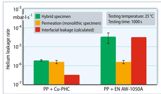
**Fig. 4.** Interfacial leakage rates minus permeation values of different polymer-metal hybrids: the PP-copper specimens show significantly lower leakage than specimens of PP and aluminum
