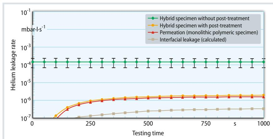
**Fig. 3.** Differentiation between permeation and interfacial leakage determined by using DTPM on thermally post-treated, adhesion-modified polymer-metal hybrids at 23 °C: thermal post-treatment of the hybrid parts clearly influences the leakage rate as well as its development over time
