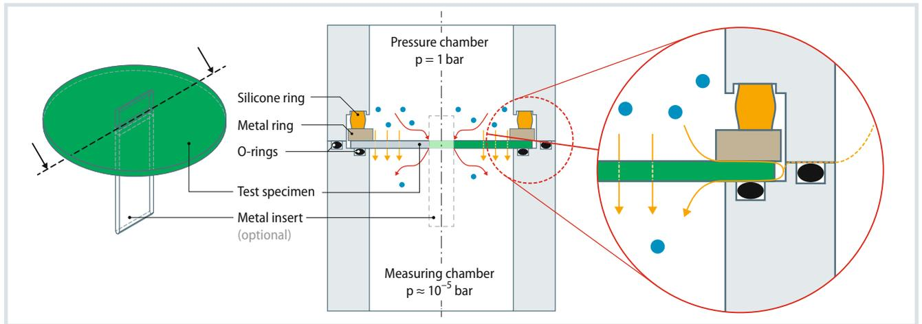
**Fig. 1.** Left: three-dimensional view of a test specimen with metal insert; right: test specimen located between pressure and measuring chamber, arrows show possible permeation paths (orange) and interfacial leakage paths (red) Source: Aalen University; graphic: © Hanser
