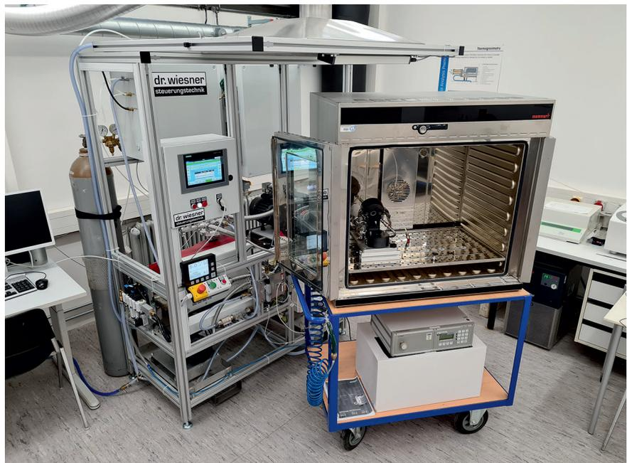
The DDP method enables more accurate determination of the tightness of polymer-metal hybrids
