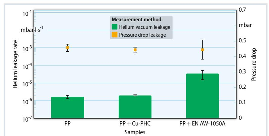
**Fig. 2.** Leakage measurement results using different measuring methods on the same samples at  $23^\circ\text{C}$  (averages from five measurements each): in contrast to the differential pressure method, clear differences in the leakage rate can be seen with the helium vacuum test
